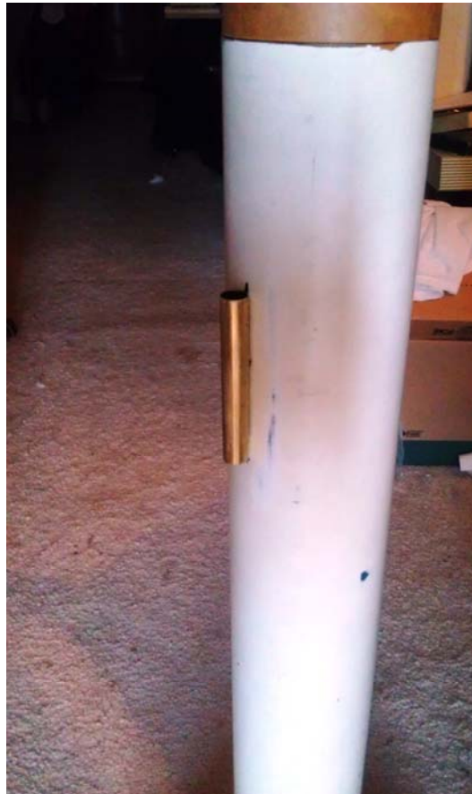
A brass launch lug is installed
