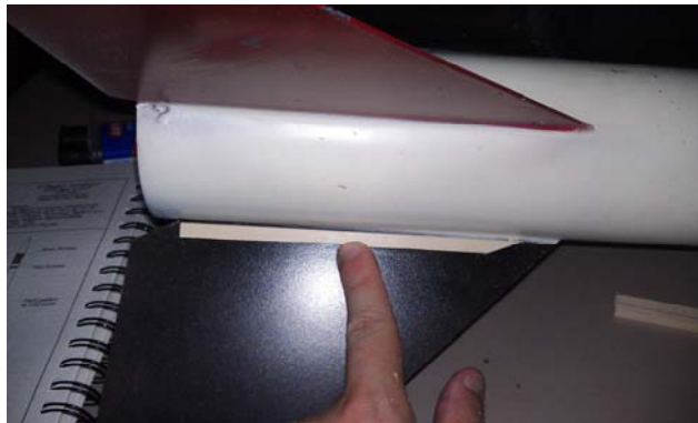
Left: Test fitting a fairing
